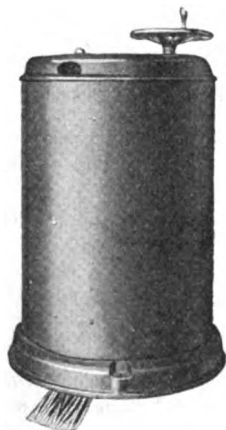
HAND-OPERATED DRUM-CONTROL SWITCH FOR VARYING VOLTAGE OF TESTING TRANSFORMERS (128 POINTS)
